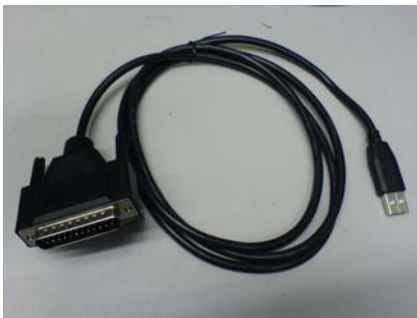
USB Connector (USB Port of PC) to DB-25 pins Parallel Connector (USB PB)
